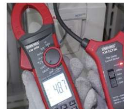
Flexible current probe (optional) to extend the AC current measurement range to 3000A
